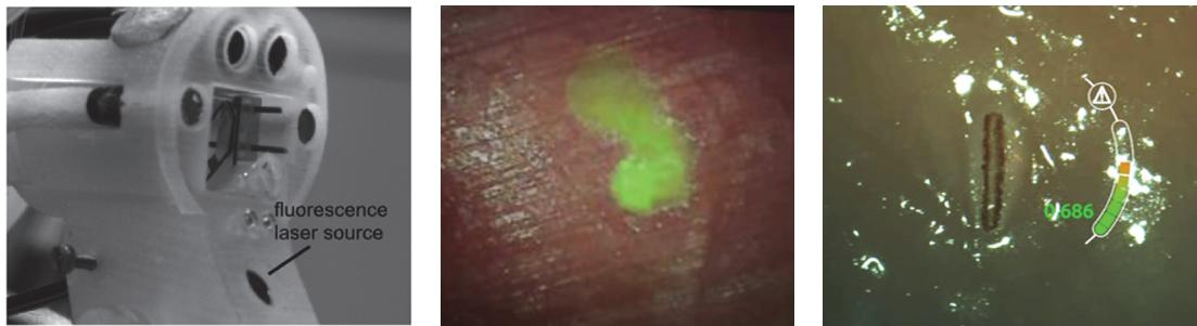
Fig. 3: Hyperspectrum fluorescence imaging system incorporated to the endoscope tip (right) and a sample image captured with the device displayed using augmented reality (center). On the right, assistive system for precise control of laser incision depth based on the cognitive modeling of laser-tissue interactions.
