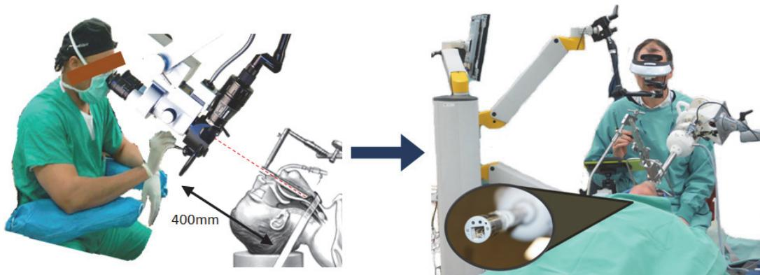
Fig. 1: The μRALP concept: from the gold-standard free-beam laser phonometric surgery (left) towards safe and accurate endoscopic micro-robot-assisted laser phonometric surgery (right).
