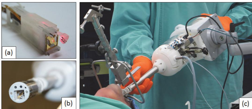
Fig. 2: Final robotics endoscope prototype incorporating: (a) Laser deflecting micro-robot; (b) multifunctional tip and flexible shaft; and (c) hybrid actuation unit.
