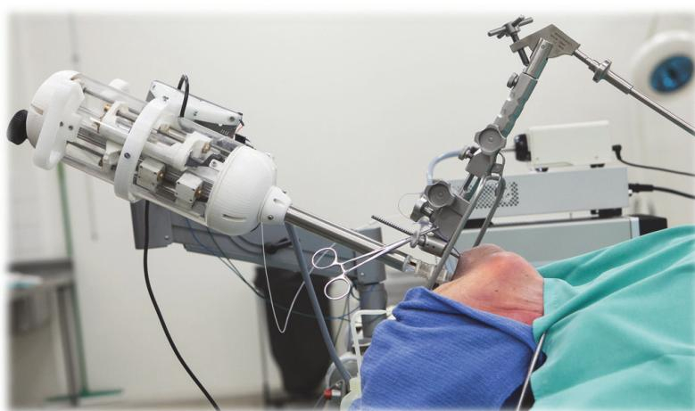
Fig. 6. The μRALP Surgical System was developed and evaluated in realistic operation conditions based on numerous cadaveric studies.
