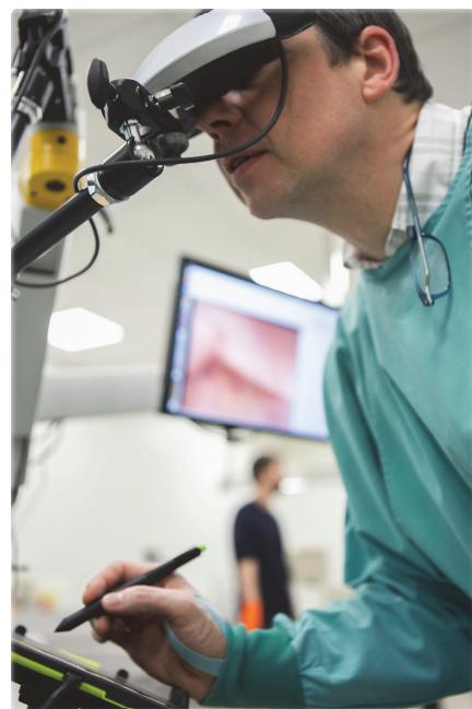
Fig. 5. Teleoperation interface: 3D endoscopic view and intuitive laser control based on a graphics tablet.
